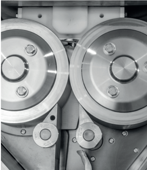
Counter-Rotating Rolls For Precise Controllable Compaction
