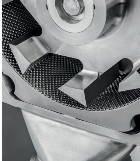
Bar Rotor For Slow-Speed “Shearing” of Compact
